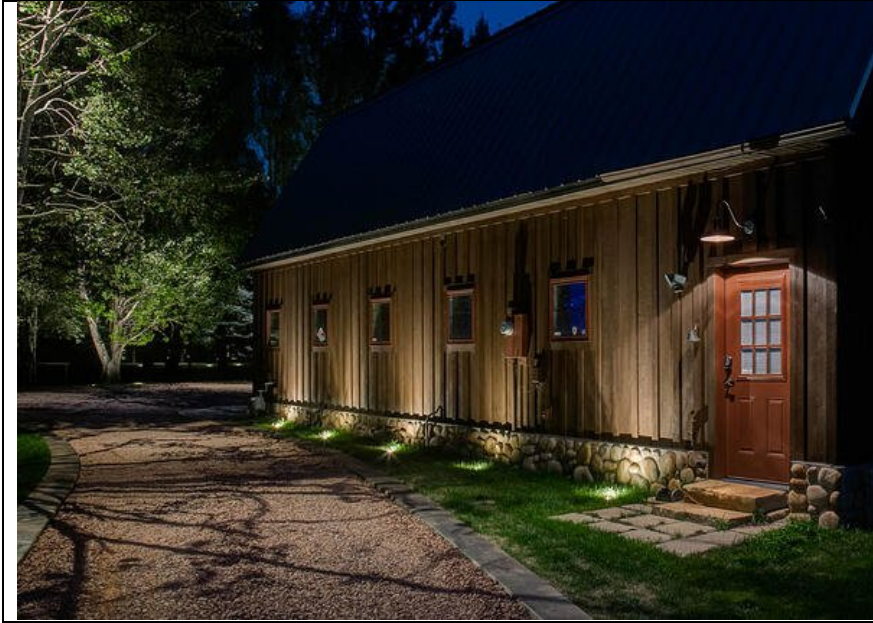
Figure 3-- A side door to a garage is an important area to illuminate, as it is often a target for break-ins.
